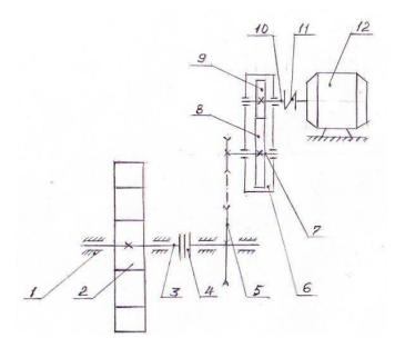
Electro-generator moving parts, chain drive andkinematics of the drive consisting of a cylindrical gear wheel and an accelerator scheme
