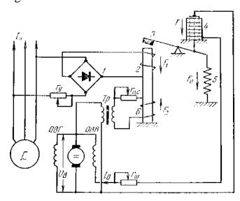
He drives a synchronous generator using a carbon rectifier automatic manage principle of the system scheme.
