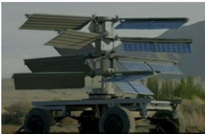
**Figure 3.** Hybrid solar-wind device with vertical axis.
