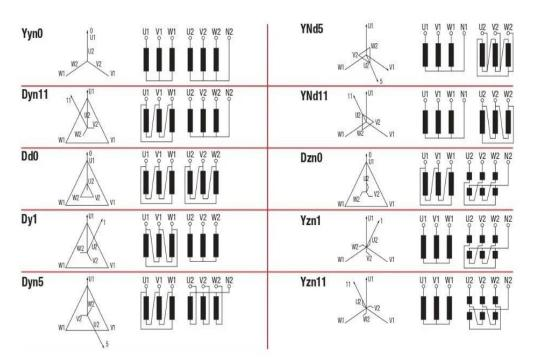
They are divided into the following four main groups according to the phase shift that exists between the line voltages on the two sides of the transformer.
