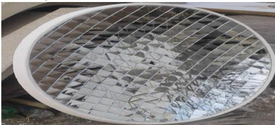
Figure 5. A real view of a paraboloid whose surface is covered with 5x5 cm mirrors.
