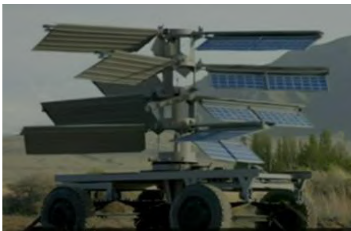
Figure 3. Hybrid solar-wind device with vertical axis.
