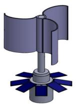
Figure 4. Hybrid solar-wind device with vertical axis.
