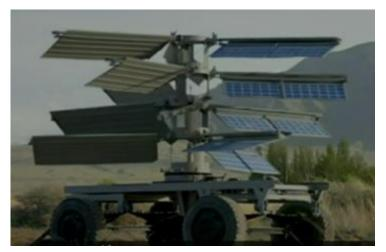
**Figure 3.** Hybrid solar-wind device with vertical axis.
