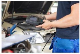
Types of diagnostic devices. All computer diagnostic systems for car shave two classifications - according to performance and functionality. In the first group, stand-alone scanners and adapters are selected. The first size is similar to a walkie-talkie, they have a display in their design and allow you to connect directly to the machine for reading information.
