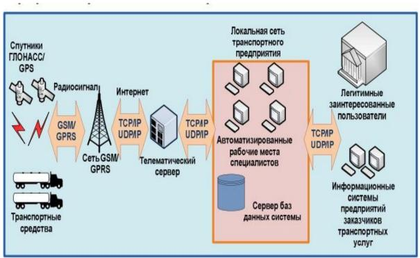
General scheme of operation of the GLONASS/GPS satellite positioning system
